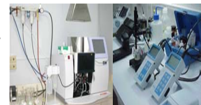
Atomic Absorption Spectrophotometer and ancillary water testing equipment
